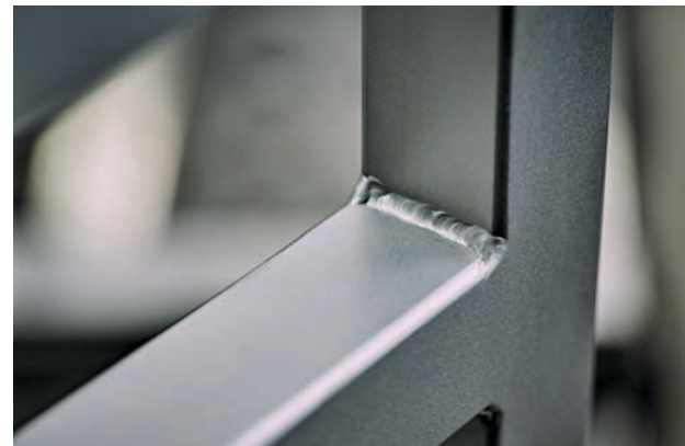
Fig. clean and corrosion resistant weld seams (TIG welding)
