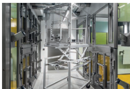
Fig. mobile capturing/ application cage for the transport of single animals
