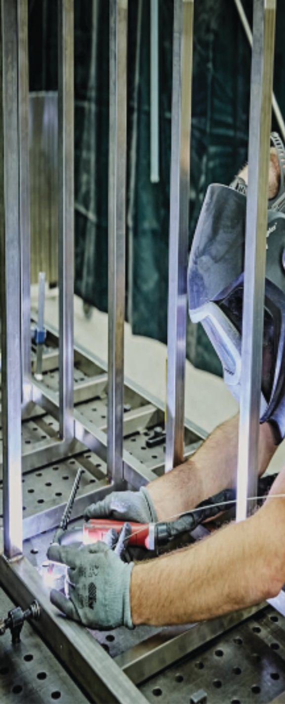
Fig. assembly production of stain-less steel components (TIG welding)
